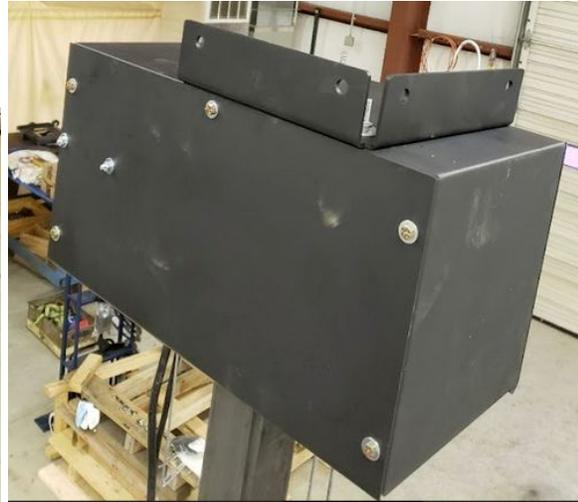
A lift with a station height over 72" requires the use of a bracket cap and will require customer provided bracing that will connect the bracket cap (and column) to an adjacent support structure, ideally a strong wall. Care should be taken to assure that the bracing is securely attached to the wall and that the wall is strong enough to withstand the expected lateral forces.
